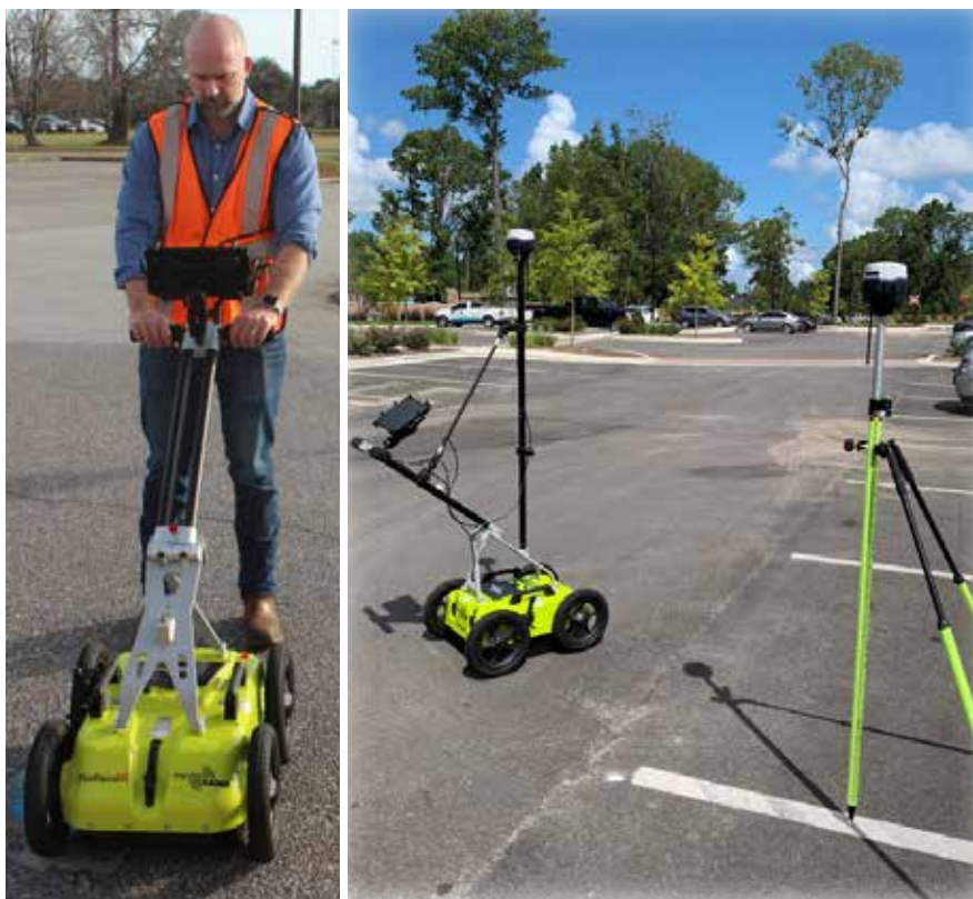
Figure 1. ImpulseRadar PinPointR GPR system configured with Emlid RTK Base and Rover.
